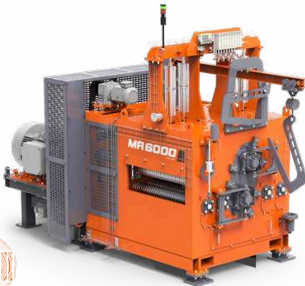
The MR6000 is Wood-Mizer's largest capacity multirip saw with the standard machine capable of processing material up to 914 mm wide and up to 254 mm thick. Featuring dual arbors, the MR6000 can be equipped with a configurable number of circular saw blades for processing material. Additional configurations for material width, thickness, and power are available based on the number of saw lines and processing needs.
