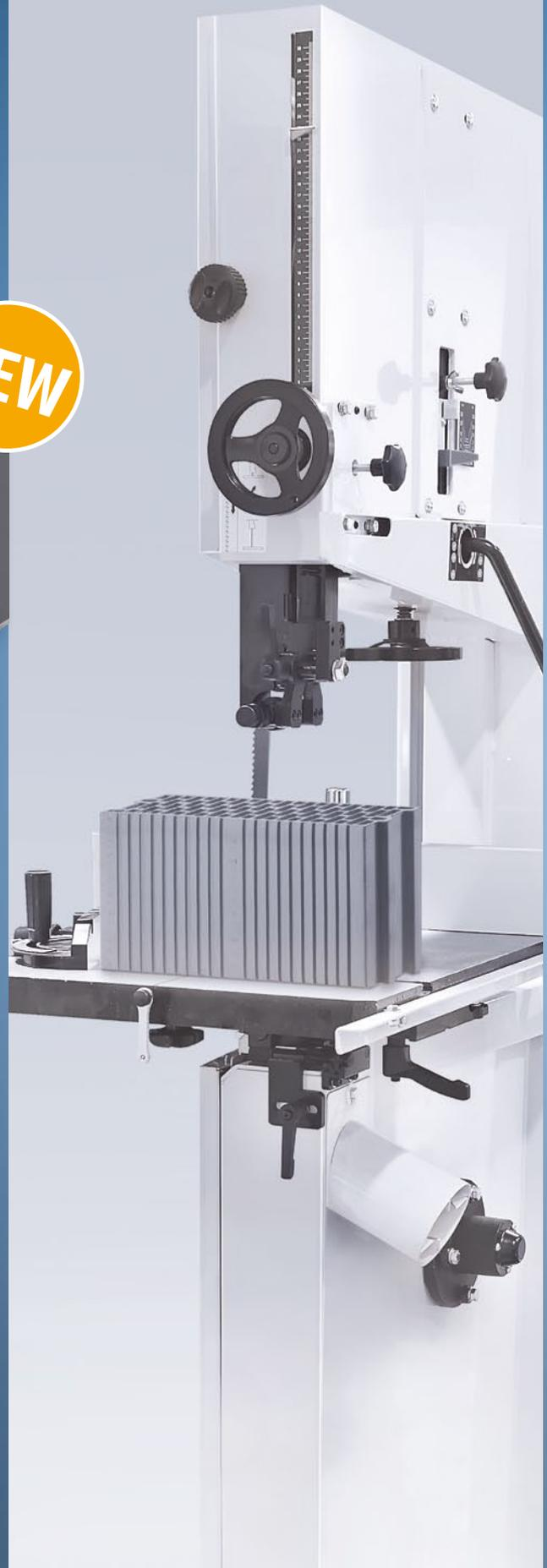
The universal band saw blade for all construction and insulation materials of small and large dimensions running on brick band saw machines.
