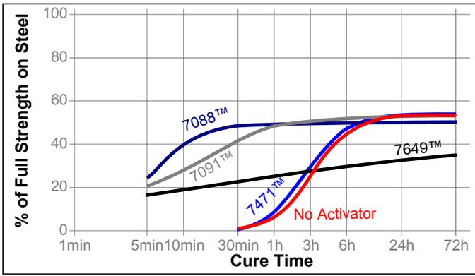
Breakloose Torque, ISO 10964, Pre-torqued to 5 N·m:
