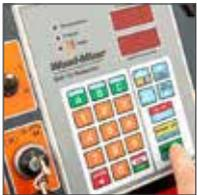
**SW10** Increases productivity using easy-to-use setworks to precisely position the head for the next cut.
