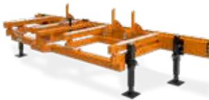
Most Wood-Mizer portable sawmills can handle just about any log length imaginable. You can add 1.8 m or 3.6 m or 7.2 m extensions to the existing bed sections, and tackle super-long logs with ease.
