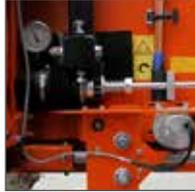
**Hydraulic Blade Tensioning**
