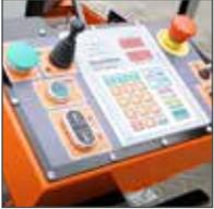
**Saw head control panel** Including SW10 Networks, forward/reverse and up/down for ease of operation.
