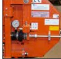
**Blade tension** is easily adjusted, and keeps the blade at the proper tension for cutting.
