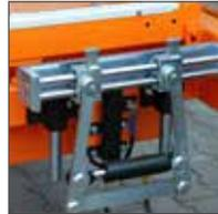
**Hold-down clamps** Invaluable when cutting logs which have compression or tension wood.
