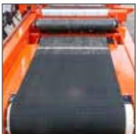
**Board Removal Conveyor** Automatically activates when board is being removed.
