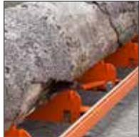
**Raised Cross Bed Sections** for easy loading of logs with a forklift or tractor.
