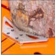
**Uniqu clamping system for irregular logs**
