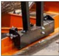
**xFrame** stable structure that travels on twin parallel steel profiles on the bed.
