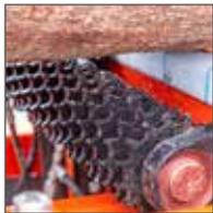
**Power Roller** easily enables you to position the log on the bedrails, and can also assist in removing sawn cants.
