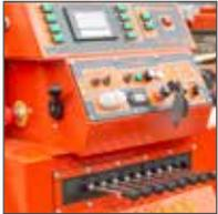
**Control Panel with Setworks** increases productivity and accurately positions the head for the next cut.
