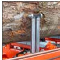
**Double Vertical Support** Provide a surface to clamp the log against, allowing the log to be cut perfectly square.
