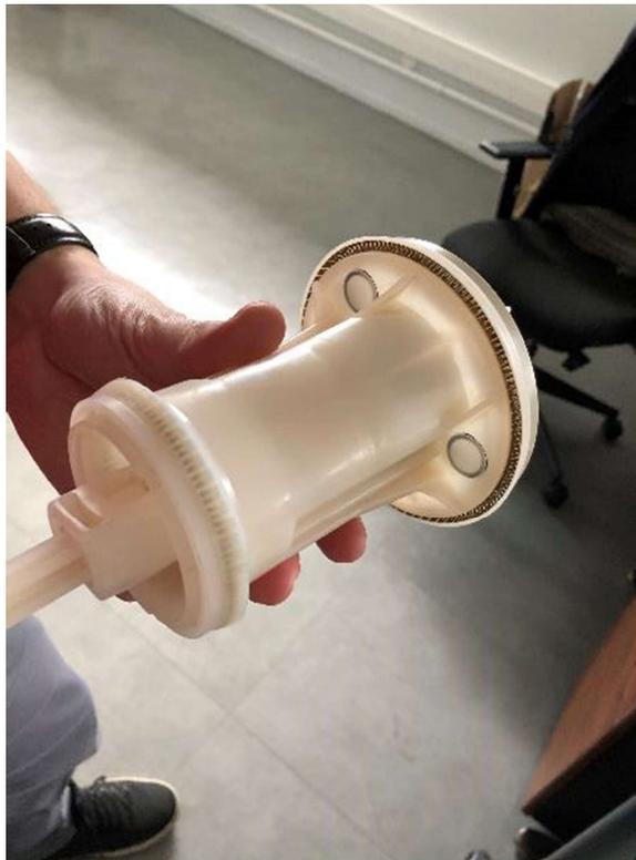
1. Make  $\frac{1}{4}$  turn in the trigonometric way to unlock the blocking ring.
