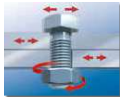
Vibration and loosening.
