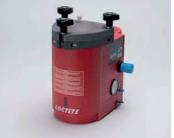
LOCTITE 97009 Integrated Semi-Automatic Dispensing System to dispense the adhesive directly from larger bottles. The controller provides digital timing control for any LOCTITE automatic dispense valve or automatic hand-held applicator. It is equipped with a precision pressure regulator, with a range of 0.1–4 bar for reliable dispensing, eliminating air pressure fluctuations.
