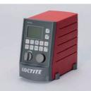
LOCTITE 97152 Dual Channel Controller is a versatile multi-functional controller for actuating 1–2 dispensing valves. Settings can be made via the membrane keypad and the rotary selector switch. Reservoir pressure is controlled via a precision pressure regulator and monitored electronically.
