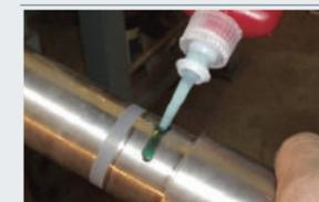
Recommended for parts that will need subsequent dismantling, i.e. retention of bearings onto shafts and into housings.
