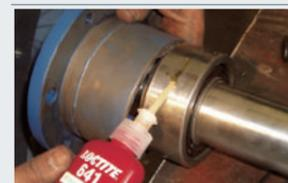
A controlled strength retaining compound that is ideal for cylindrical parts that require disassembly.
