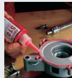
High temperature. Product has a temperature range to 400°F (204°C) with excellent solvent and chemical resistance. Makes or dresses gaskets in rigid assemblies. Eliminates gasket compression set.
