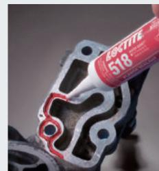
Recommended for use on rigid iron, steel and aluminum flanges. Spray LOCTITE® 7649 Primer N on only one surface.
