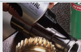
Used for repairing worn coaxial parts without remachining; enables reuse of worn bearing seats, keys, splines, tapers, or for retaining shims.
