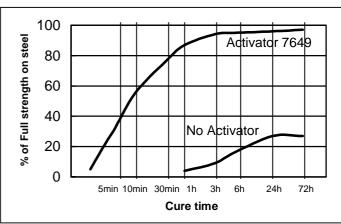
The graph below shows the breakaway torque strength developed with time at 5 °C on M10 mild steel nuts & bolts and tested.
