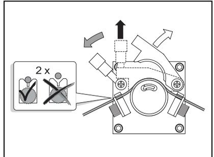
The tube is guided and held in place with the tube holder **13**.
